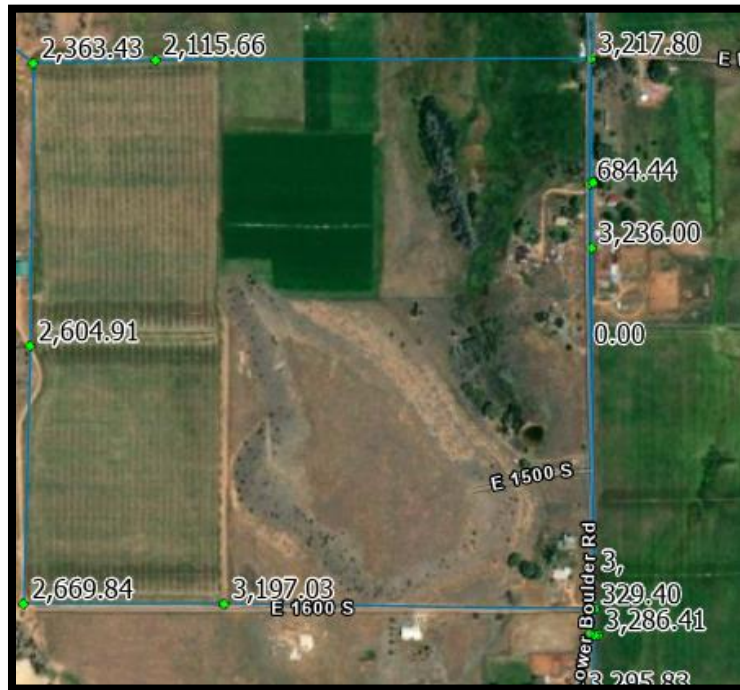
Figure 6 Alt 2 Fire Flow Capacity
