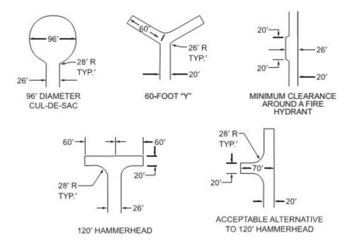
Since all our equipment is smaller the cul-de-sac could be 80' diameter instead of 96' and the hammerhead or "Y" could have 50' length instead of the 60' or 70' in the image.
